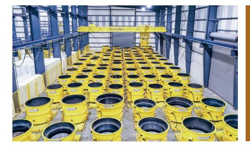
Flexible production plants from Schlüsselbauer, which offer impressive efficiency and overall performance, are now in use around the world. Highly automated plants for the production of custom-fit Perfect manhole bases and more components manufactured using the wet cast process are being installed by Ameritex Pipe & Products at two locations in
