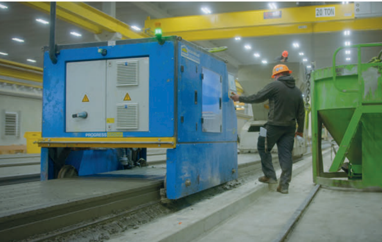
With the Automatic Plotter SmartJet it is possible to draw and print data on the precast concrete elements.
