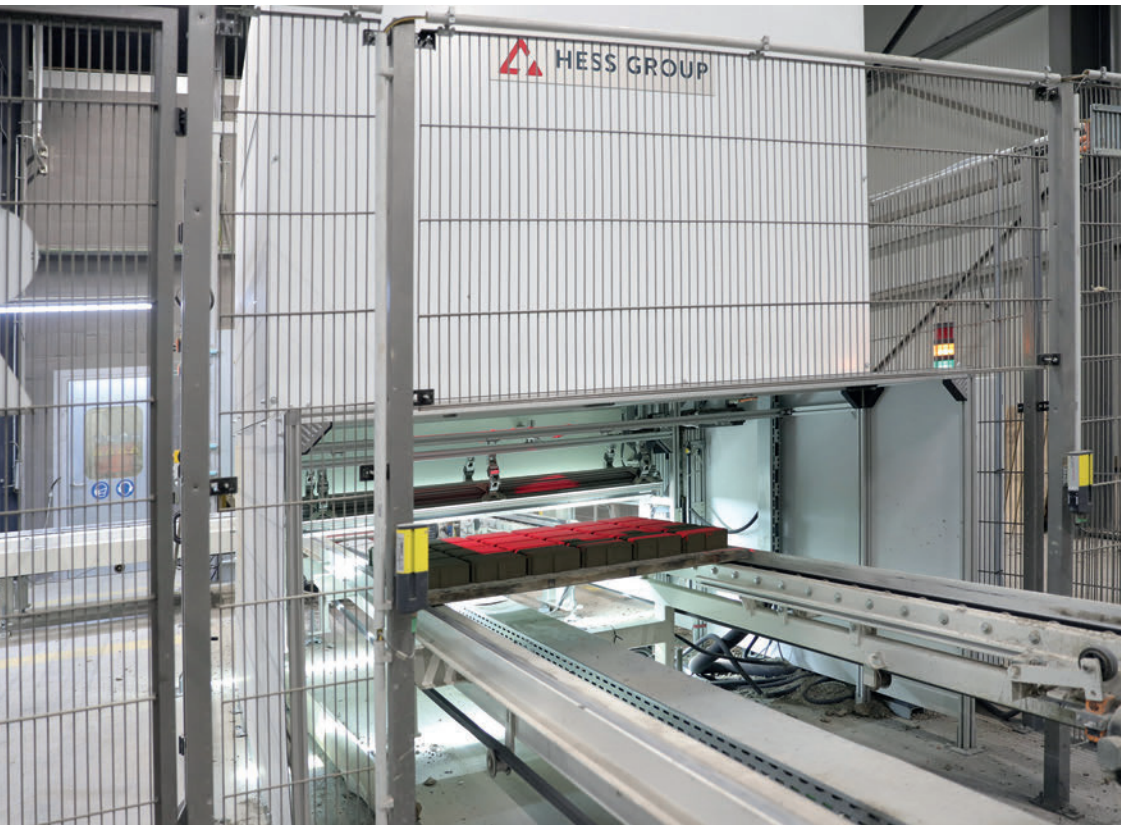
Inline QC - prototype of the camera system on the wet side
