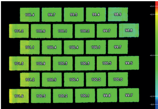
The color indication in the relief can be used to quickly and easily determine the different heights over a measured layer of product.
