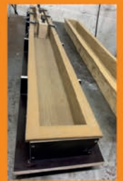
Ranch Post & Rails from client manufacturing concrete using Numold moulds
