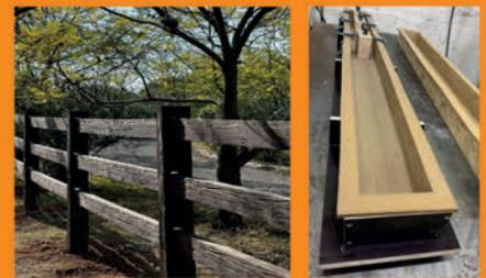
Ranch Post & Rails from client manufacturing concrete using Numold moulds
