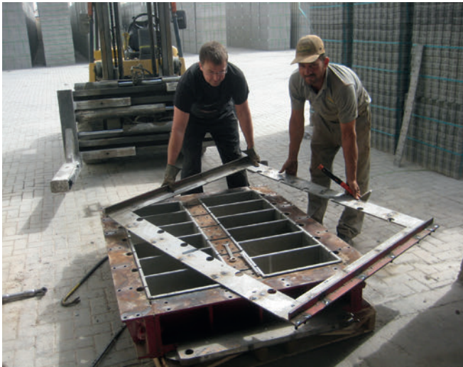
Kobra service for changing wearing parts on site
