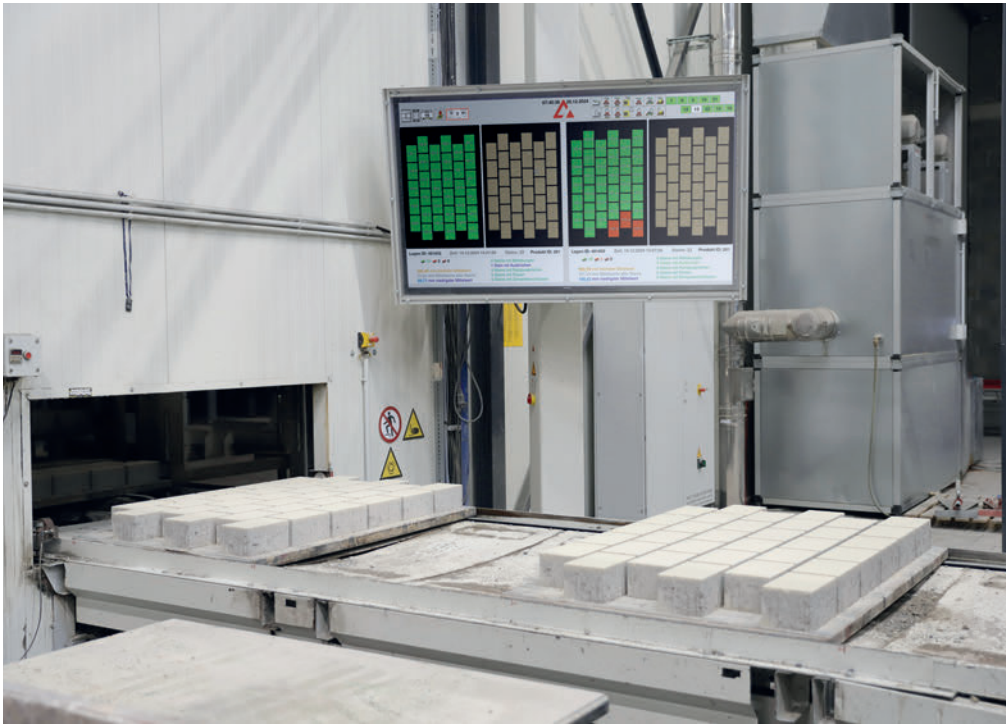
Inspection of the blocks using the Inline QC on the dry side
