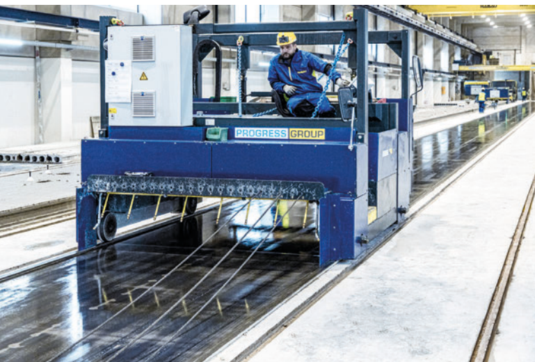
The battery-powered multifunctional trolley is used to set up a (new) line: for cleaning, oiling and pulling the strands/wires.
