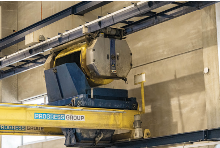
The concrete spreader with bridge is designed for the automatic supply of fresh concrete via a bucket conveyor.
