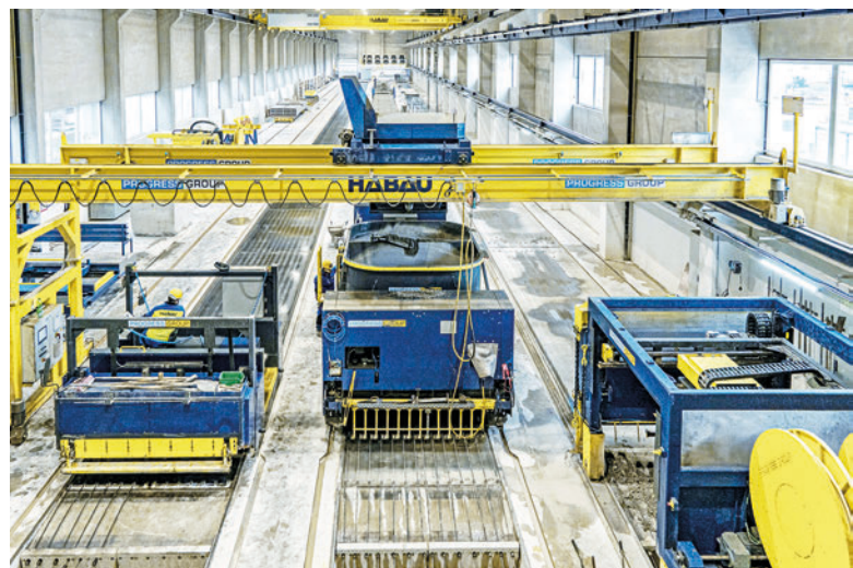
The 2.40 metre wide lines make a wide variety of products possible - for example, two 1.20 metre wide slabs can be produced in parallel on one line.
