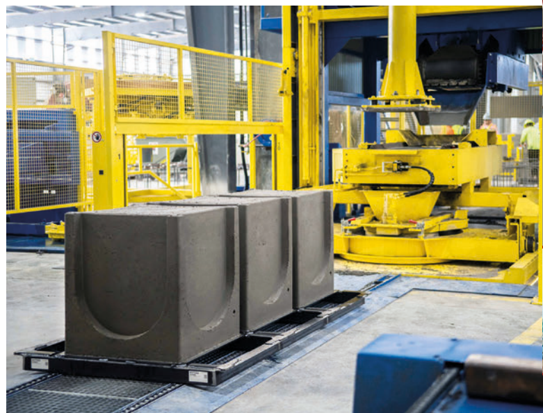
Stable bottom pallets for immediately demoulded rectangular manhole bases
