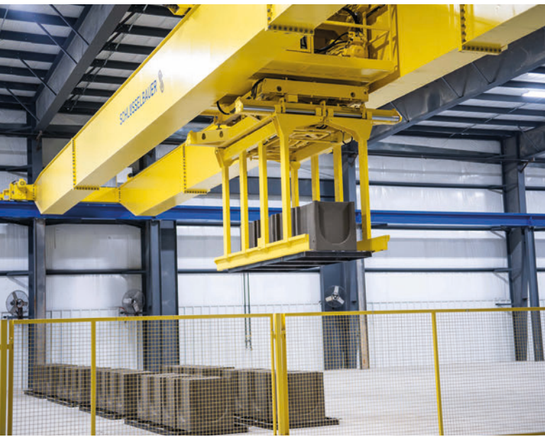
Transexact automatically transports fresh products to the curing area
