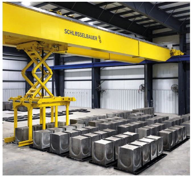
Hardened products are removed from the curing area
