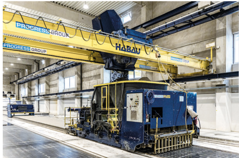
Thanks to its specific design and the use of earth-moist concrete, the S-Liner® slipformer is considered cost-efficient, easy to operate and easy to maintain.
