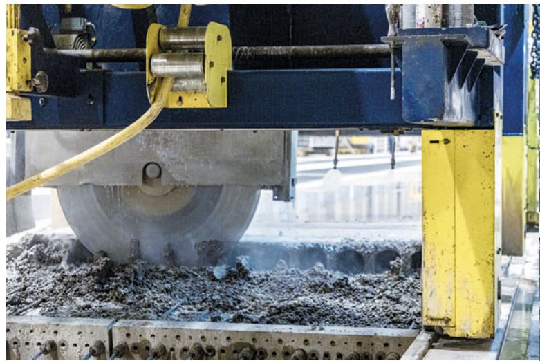
The rail-guided sawing machine produces clean, precise cuts in hardened concrete elements and fresh concrete.
