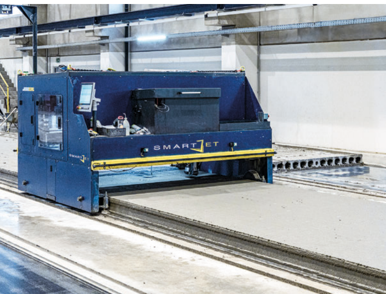
In addition to the printing device, the SmartJet plotter is equipped with an additional drilling device.
