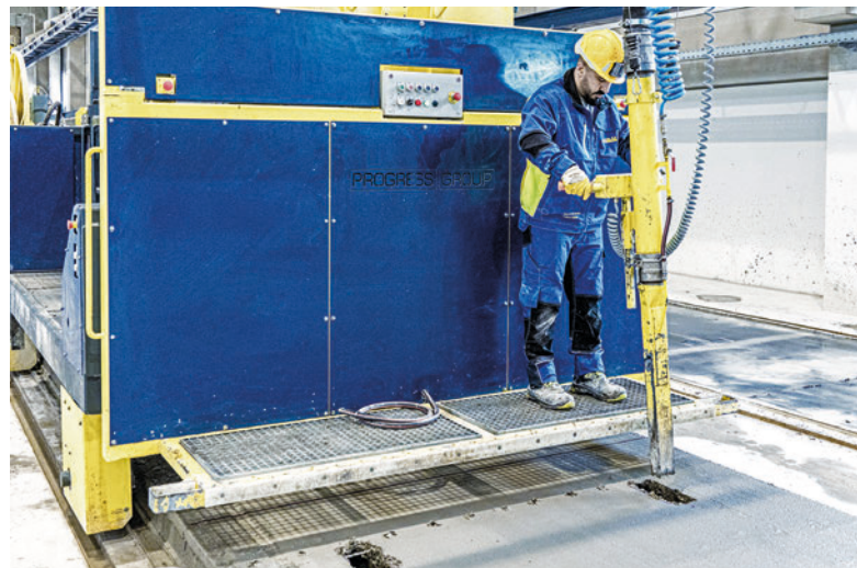
The concrete extraction machine is primarily used to remove concrete from recesses and openings.
