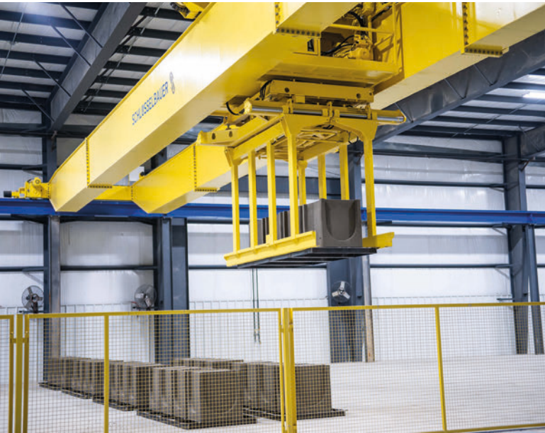
Transexact automatically transports fresh products to the curing area
