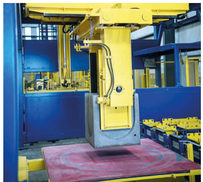
Fully automated handling (gripping, lifting, turning, setting down) of the products in the palletizing system
