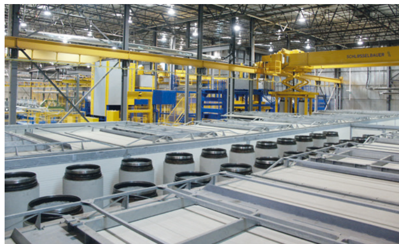
Fully automated concrete pipe production with the Exact 2500 and its steel top pallets for precise, leak-tight pipe joints.
