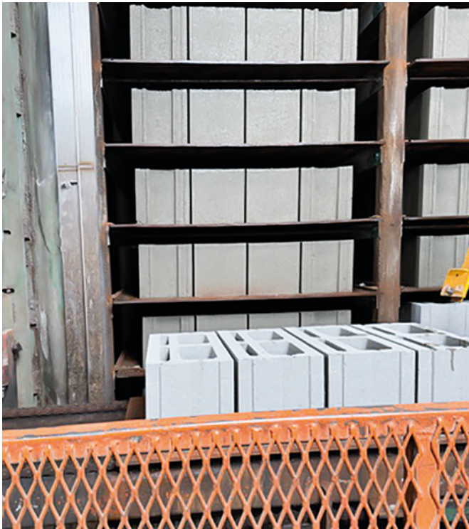
Drastic Color Difference Between the Green Blocks and Cured Blocks
