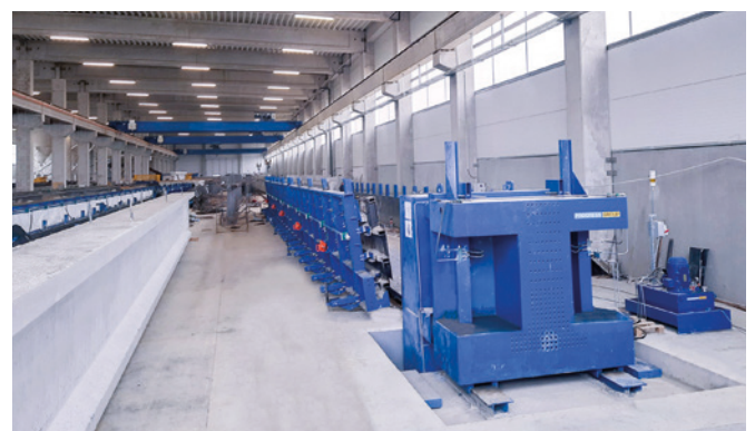
The mould for beams with abutments makes it easier to produce exactly according to the needs of the customer.
