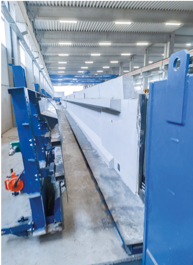
The extremely adjustable mould for I beams is 32 meters long and can produce high quality beams for medium and large industrial buildings.
