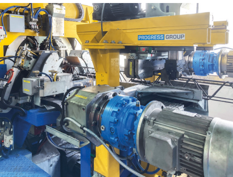
The Versa lattice girder welding machine can switch to a different lattice girder height within seconds while production is running.
