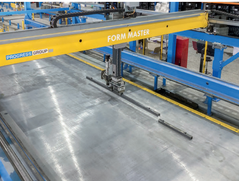
The Form Master shuttering robot lays the shuttering fully automatically according to the CAD plan.
