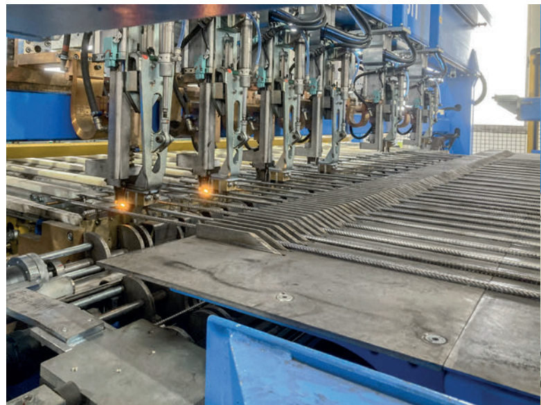
With the M-System BlueMesh® mesh welding plant, mesh and cages can be produced fully automatically from the coil in a short time.
