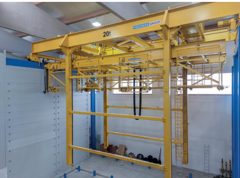
The storage and retrieval machine stores the pallets with the freshly concreted elements in the drying chamber, which now enables the precast concrete elements to cure efficiently.
