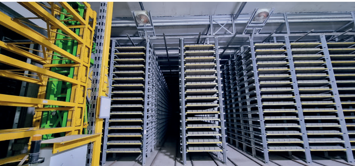
Uniform curing up to standard strength in the Rotho climate chamber
