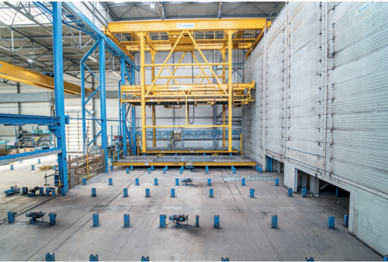
The automatic control unit transports the elements for effective curing, supported by the Green Code Curing Control.
