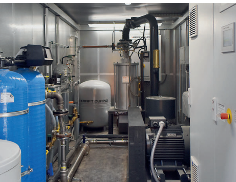
The fully kitted containerized Vapor Curing Unit.
