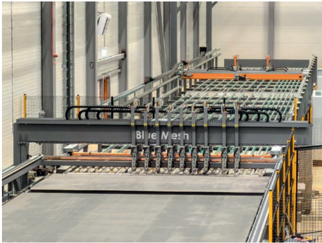
M-System mesh welding plant is welding but also bending the steel and forms them into the special cages needed.
