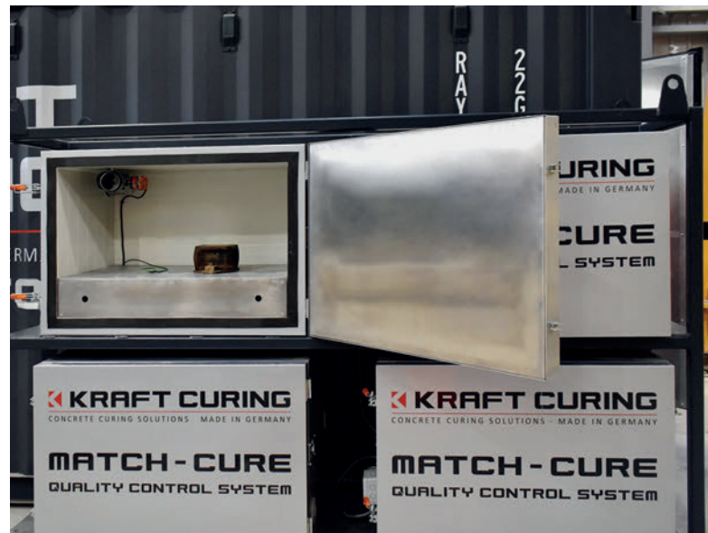
The four Match-Cure ovens located next to the containerized Vapor Generator
