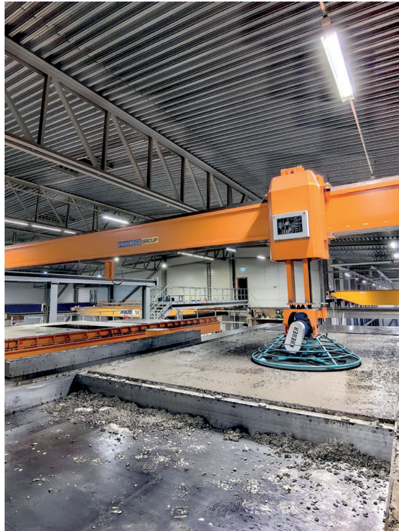
For a smooth concrete surface, the freshly poured and compressed concrete must be scraped off with the smoothing equipment.
