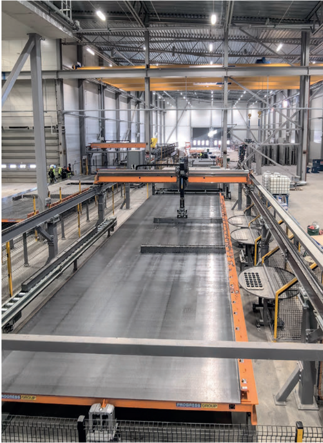
The Form Master shuttering and deshuttering robot even implements the little parts needed into the form fully automated.
