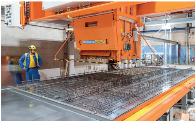
The eCon Drive concrete spreader in the factory in Ucklum can produce 5 pallets per hour with 28 m 2 per pallet.
