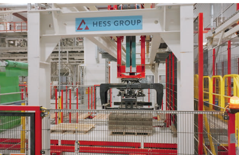
Hess Cuber efficiently transfers product layer from production board to shipping pallet cube.
