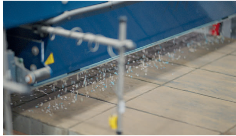
Beader device spreads a protective layer of organic beads to prevent surface damage during shipment.
