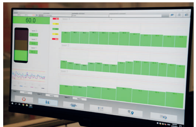
Laser measurement monitor tracks each cycle for height tolerance.
