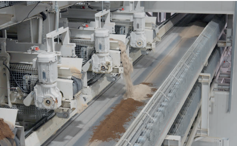
Quad Belt oscillate distribution automatically programmed for consistent color blending.
