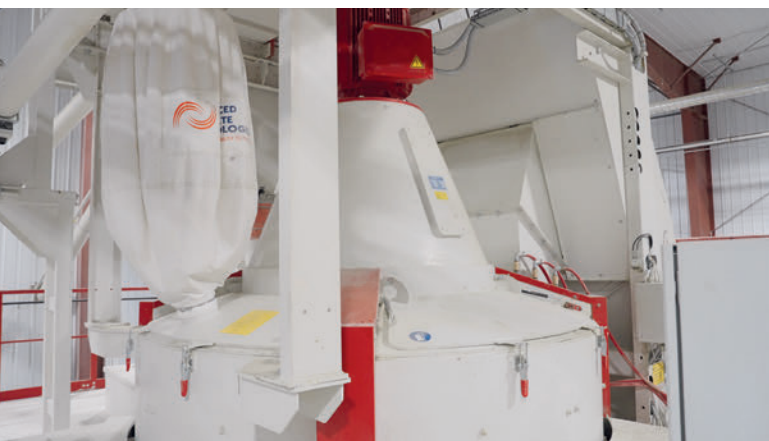
HPGM-3750 base mixer to assure constant supply for production machine.
