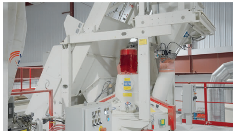
HPGM-375 face mixer for optimal mixture of finer aggregate material.
