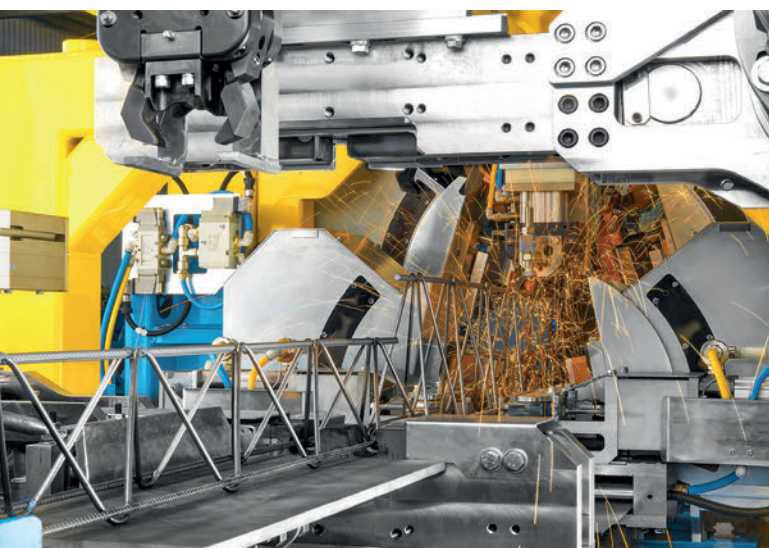
The Versa lattice girder welding machine enables flexible just-in-time production of lattice girders from coil with automatic height change.
