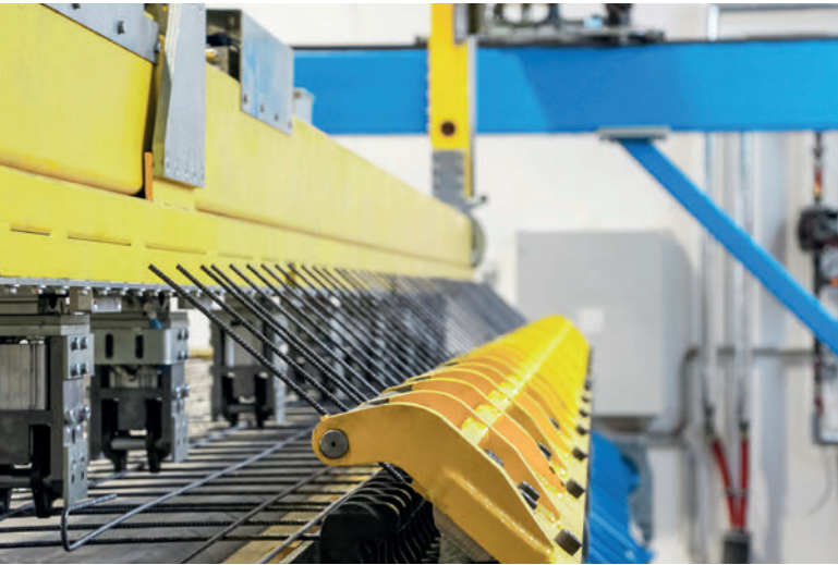
The fully integrated beam bender facilitates the processing of the flexibly produced reinforcement meshes.
