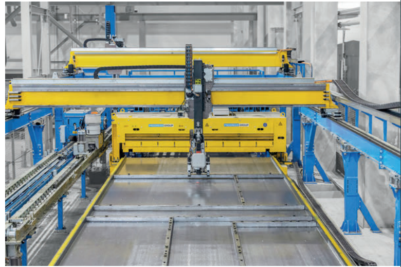
The Form Master shuttering and deshuttering robot carries out all work steps of the shuttering process fully automatically.
