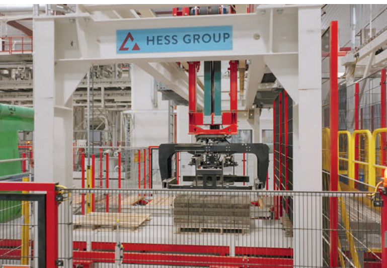
Hess Cuber efficiently transfers product layer from production board to shipping pallet cube.
