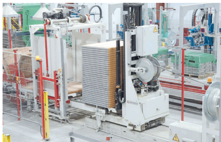
The board buffer cart automatically collects, stores, and transfer production board to machine on demand.
