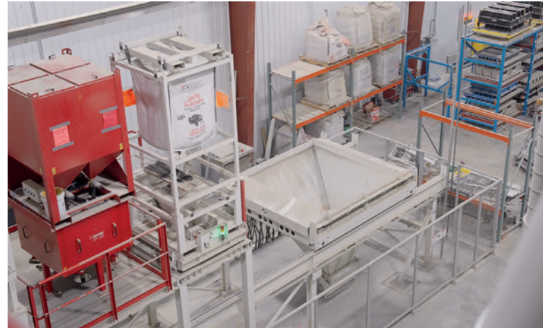
Microdoser dispenses color in grams for precise control of final color design.
