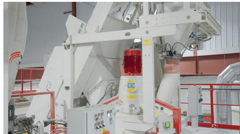
HPGM-375 face mixer for optimal mixture of finer aggregate material.
