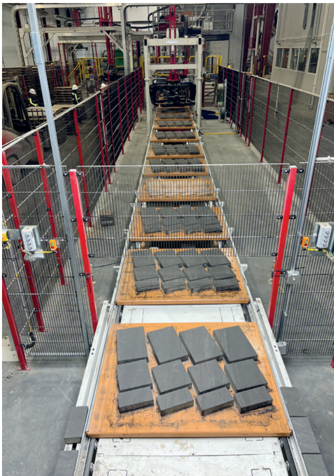
Production boards with tilted paver configuration
