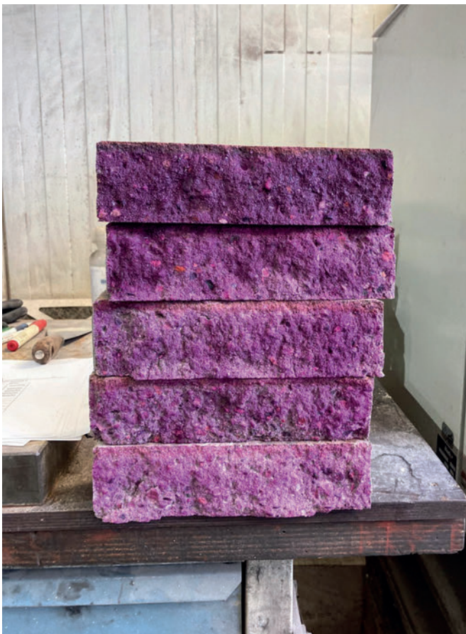
Products wetted with phenolphthalein indicator.
