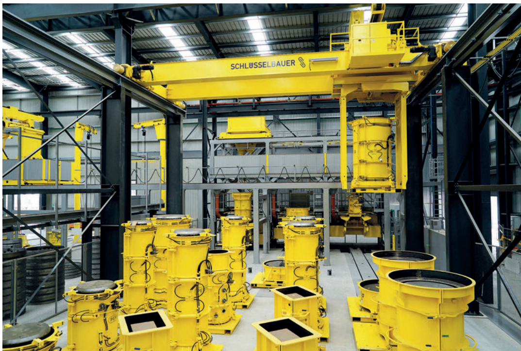
A wide variety of moulds for cost-effective mass production of wet cast components
