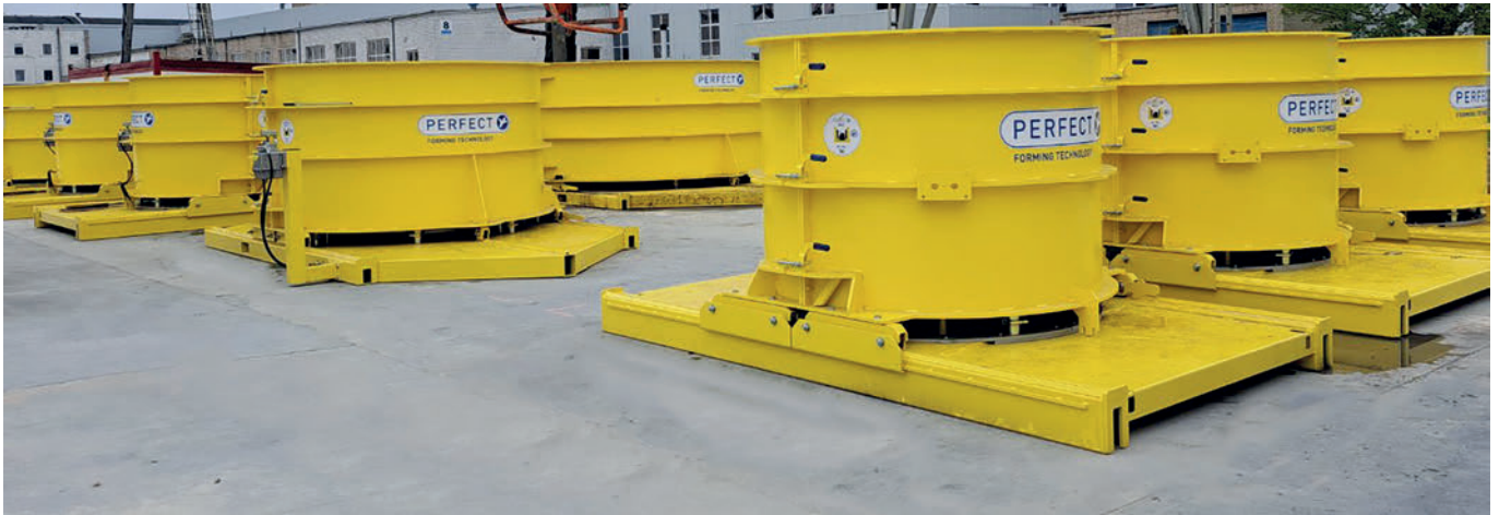
The Perfect Forming Technology concept used here for components up to an internal diameter of 3000 mm
