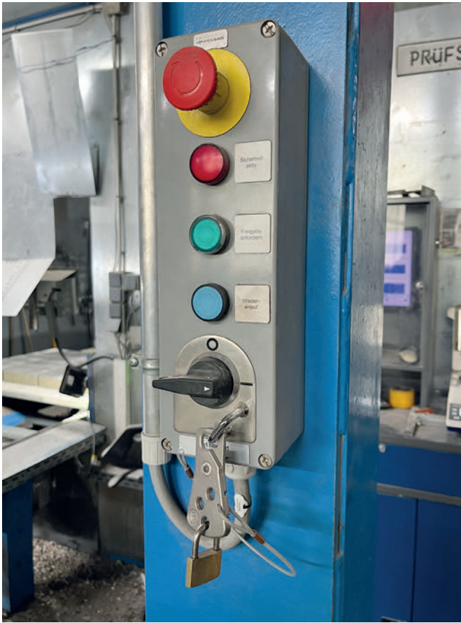
Safe and practical: Lockout-Tagout maintenance protection
