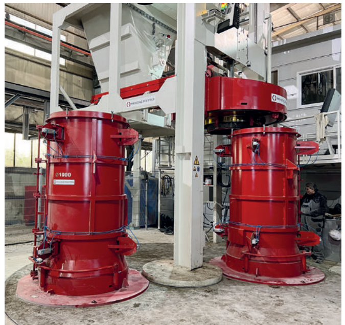
Pipe production with two moulds
