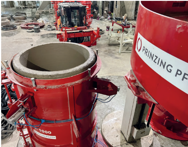
Dimensionally accurate spigot end
