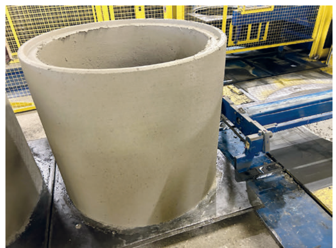
The fresh product is lifted out of the machine on the bottom pallet
