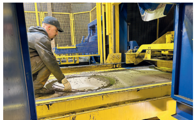
Inserting the reinforcement ring during manhole riser production
