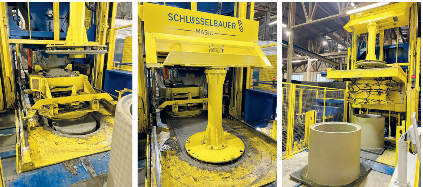
Production of a manhole riser with the Magic 1501
