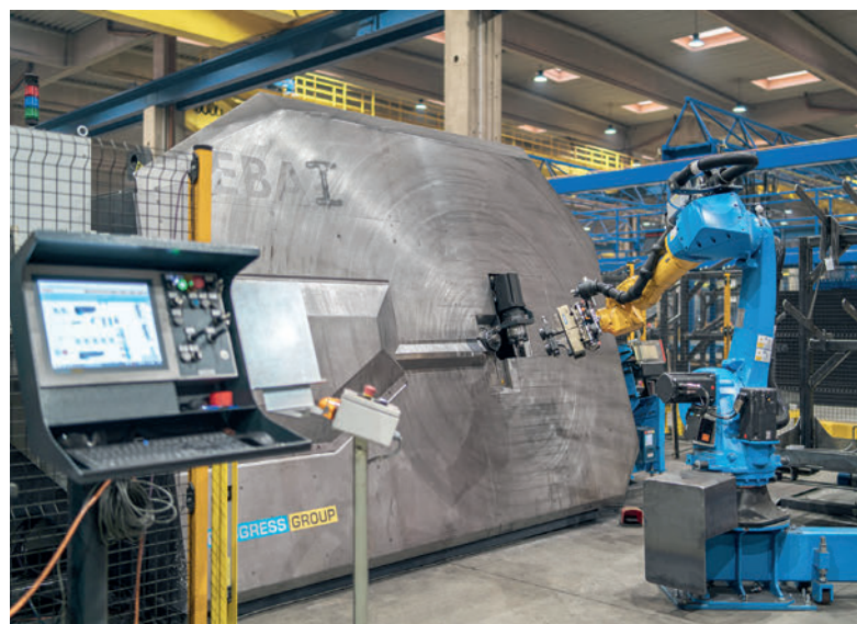
The three EBA automatic stirrup bender can cover diameters from 6 to 16 mm. One machine has a 3D bending device for the production of three-dimensional stirrups.
