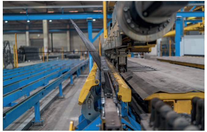
The beam bending system can automatically change the bending dies during ongoing production.
