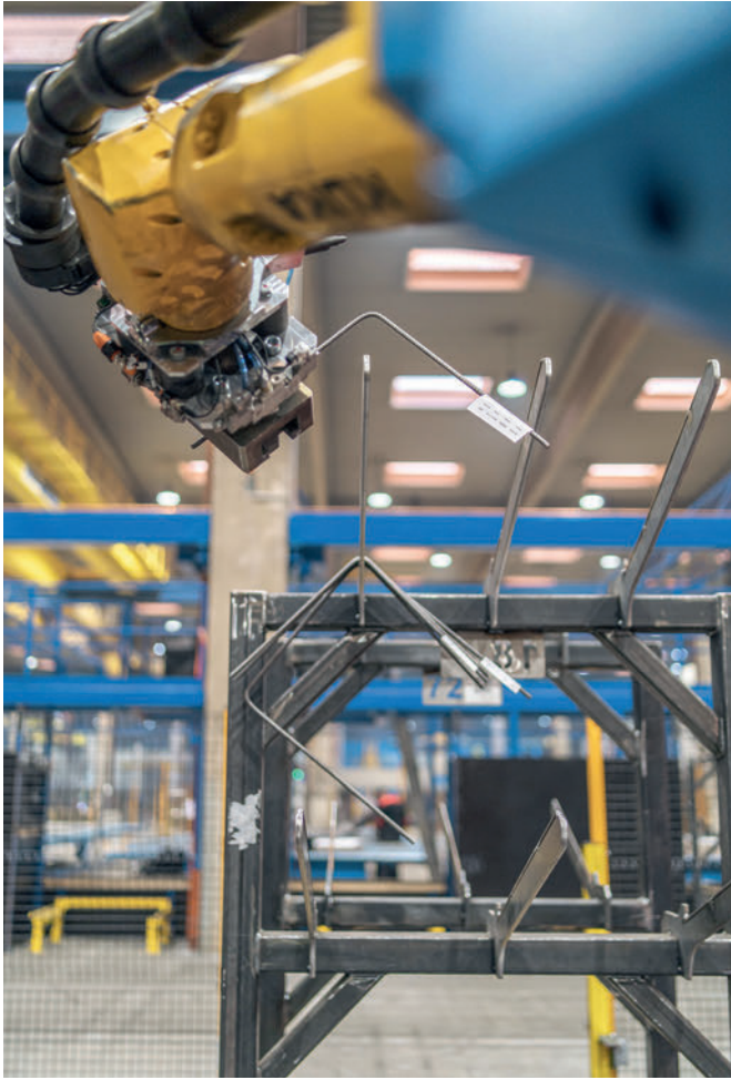
The removal robots automatically place the stirrups in the assigned position on the transport rack.
