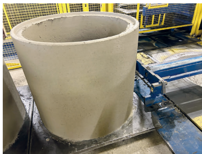
The fresh product is lifted out of the machine on the bottom pallet
