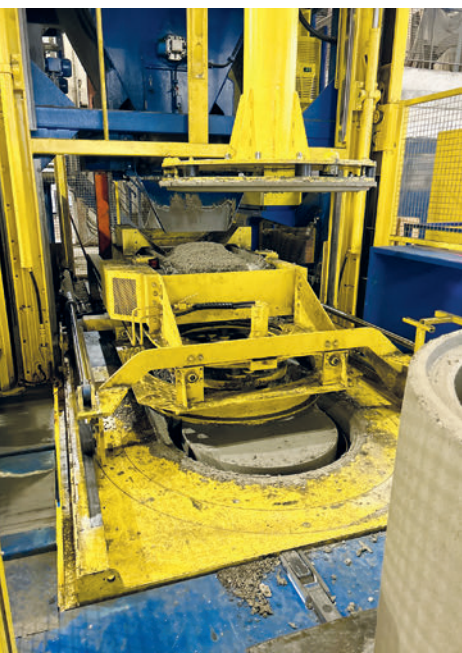
Production of a manhole riser with the Magic 1501
