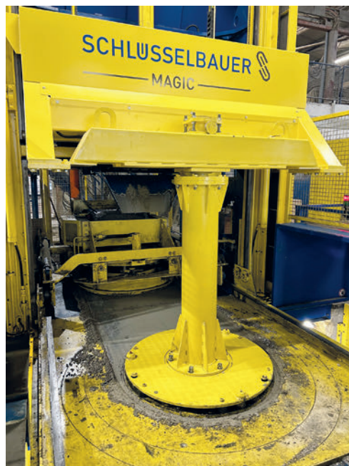
Production of a manhole riser with the Magic 1501
