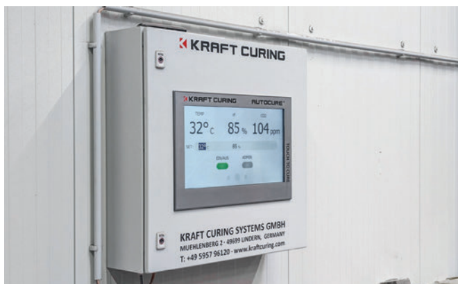
AutoCure® Accelerated Concrete curing chamber control screen
