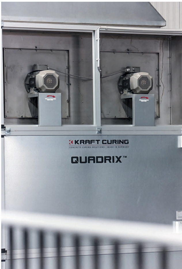
The Quadrix curing system accelerates the curing process through the controlled addition of heat and moisture
