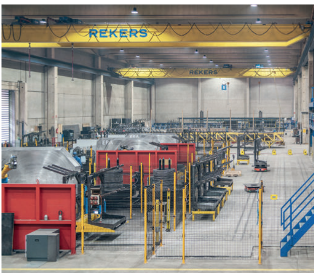
Three automatic stirrup bending machines including automated logistics were put into operation at the headquarters in Spelle.
