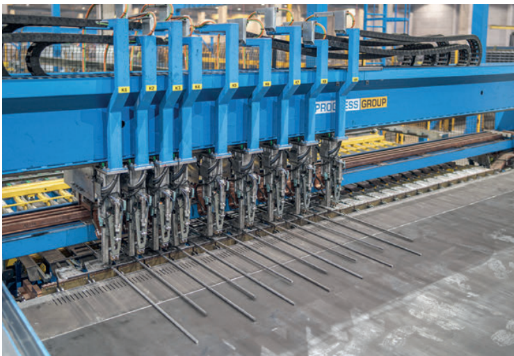
The new M-System mesh welding machine with a total of 9 welding heads ensures flexible mesh production.
