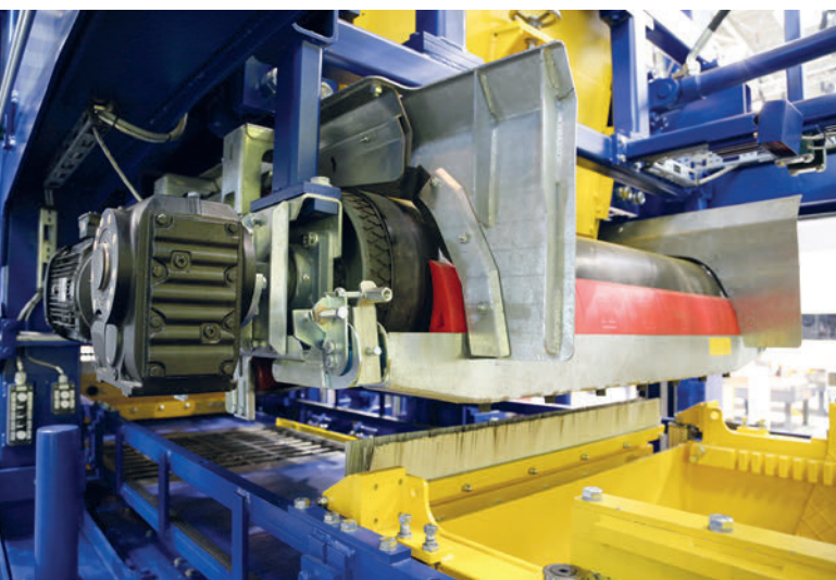
Dosing belts enable variable and optimal filling of the main and face mix filling box
