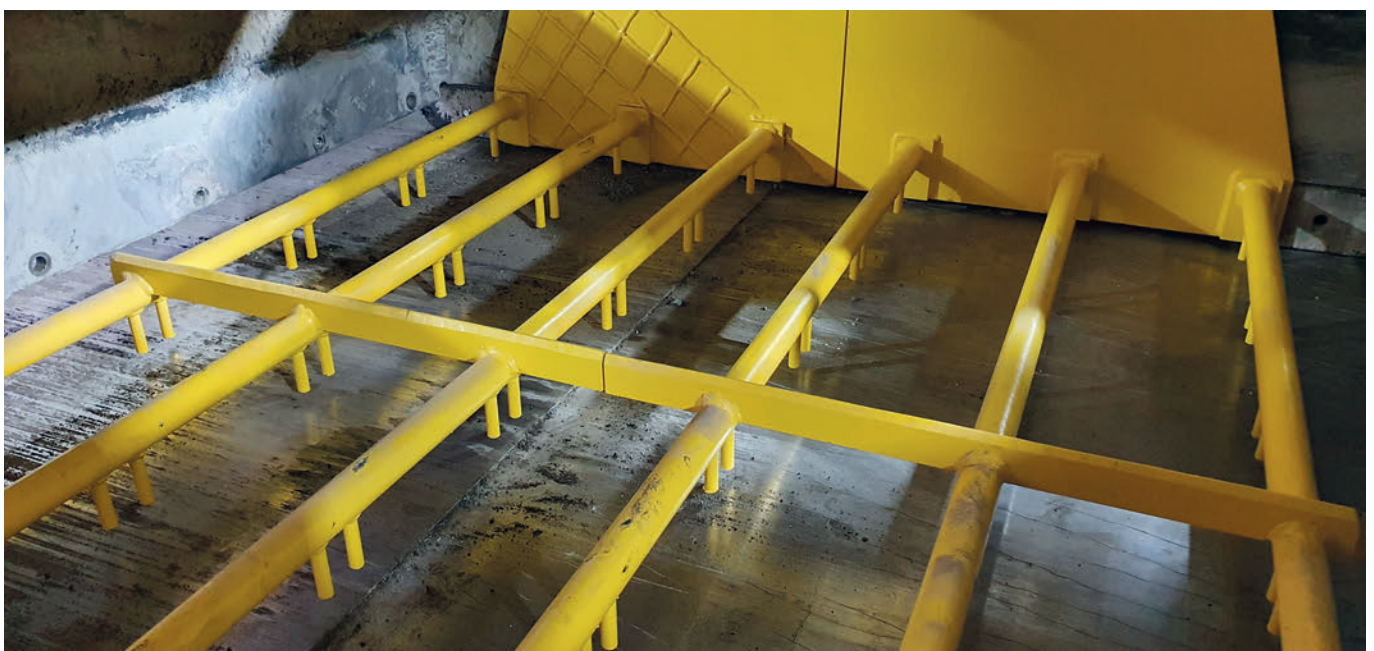
Product-specific oscillating grate insert
