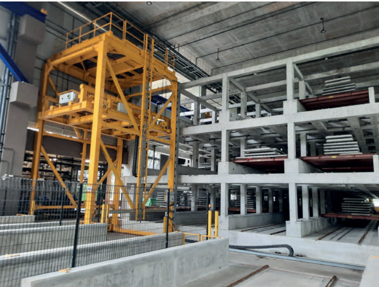
The big inside storage is equipped with an efficient storage and retrieval system - the standardized products can be stored easily.
