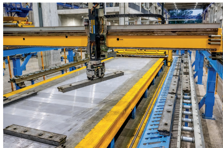
With the Form Master shuttering and deshuttering robot the shutters are placed and removed according to the provided data.
