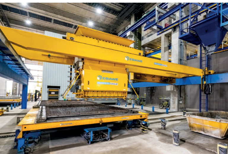
The concrete spreader is providing the exact amount of concrete needed for the element according to plan, which reduces waste.
