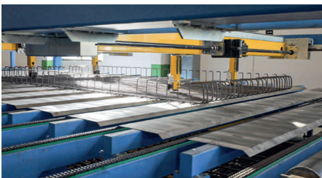
The fully automated bending solution ensures a high quality of the reinforcement cages.
