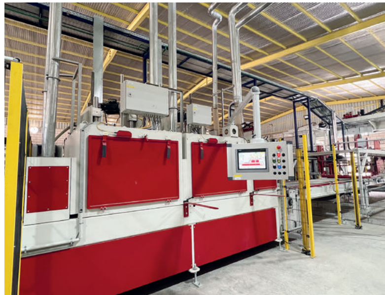
Curling machine with operation panel
