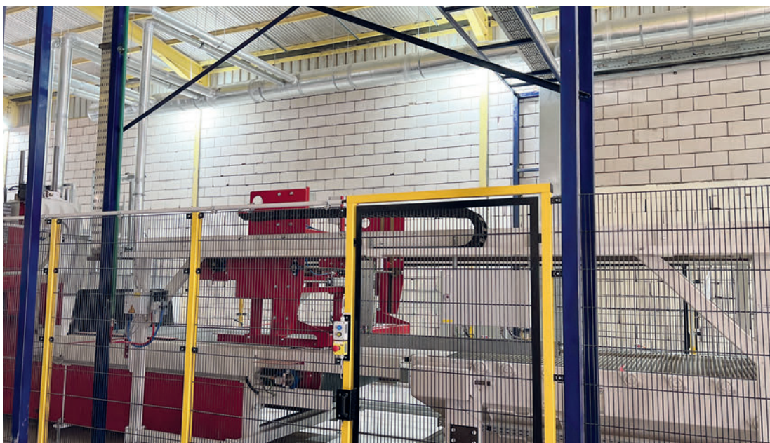
Layer pusher and retarder roller conveyor
