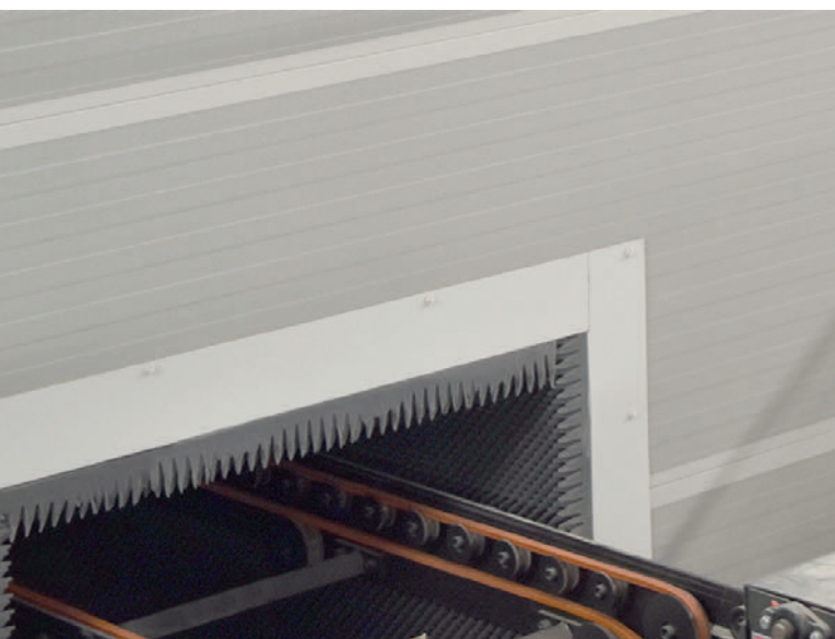
All inlet and outlet tunnels are sound insulated to reduce sound released into the production area as much as possible.
