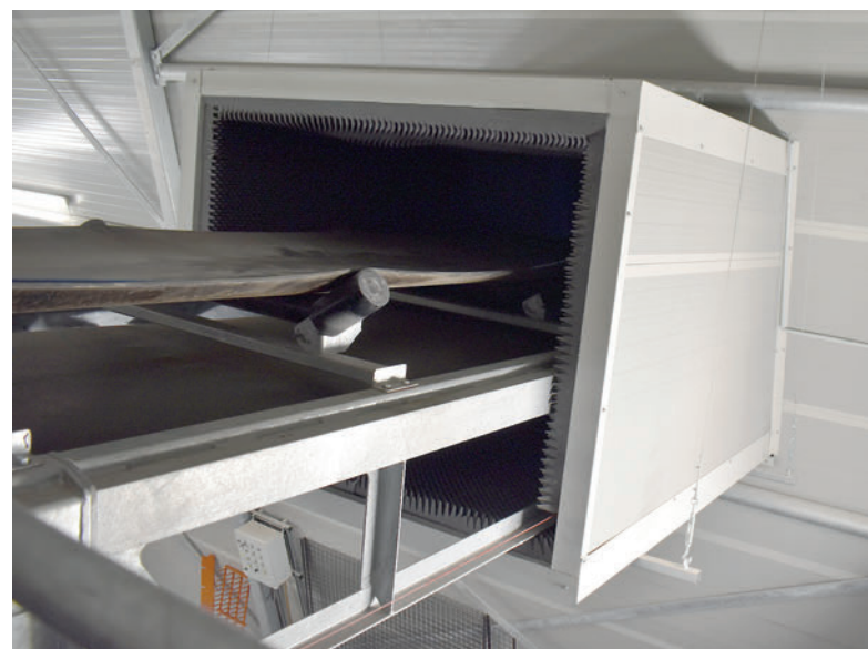
All inlet and outlet tunnels are sound insulated to reduce sound released into the production area as much as possible.
