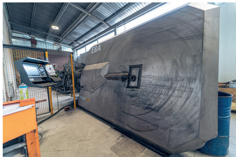
The EBA automatic stirrup bender produces stirrups in various shapes and sizes.
