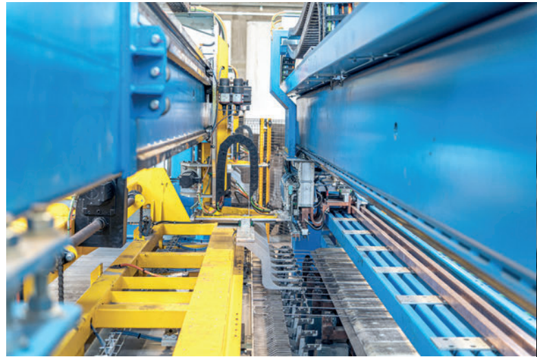
The possibility of welding longitudinal bars both at the top and bottom is an innovation developed for Prefabbricati LP.
