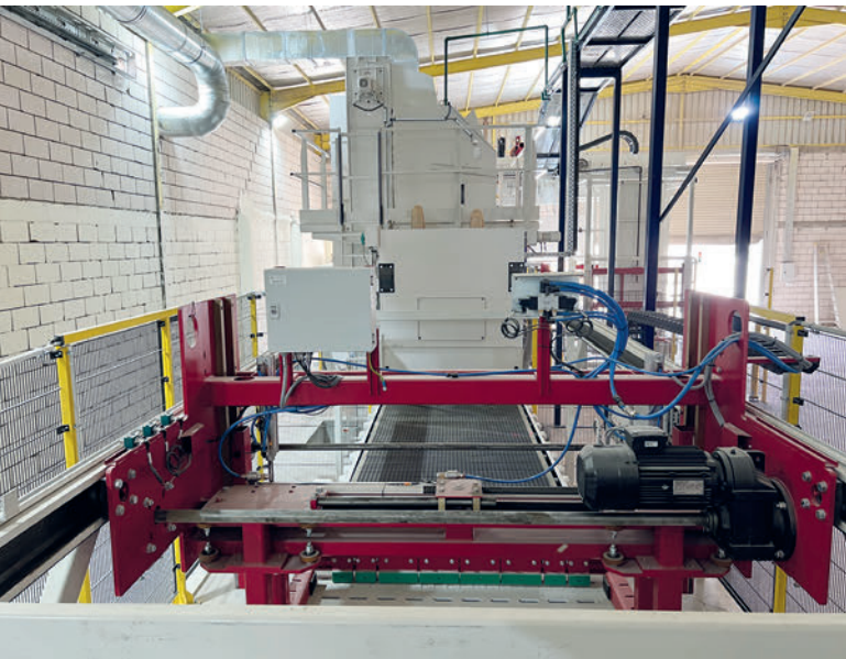
Shotblaster with layer pusher
