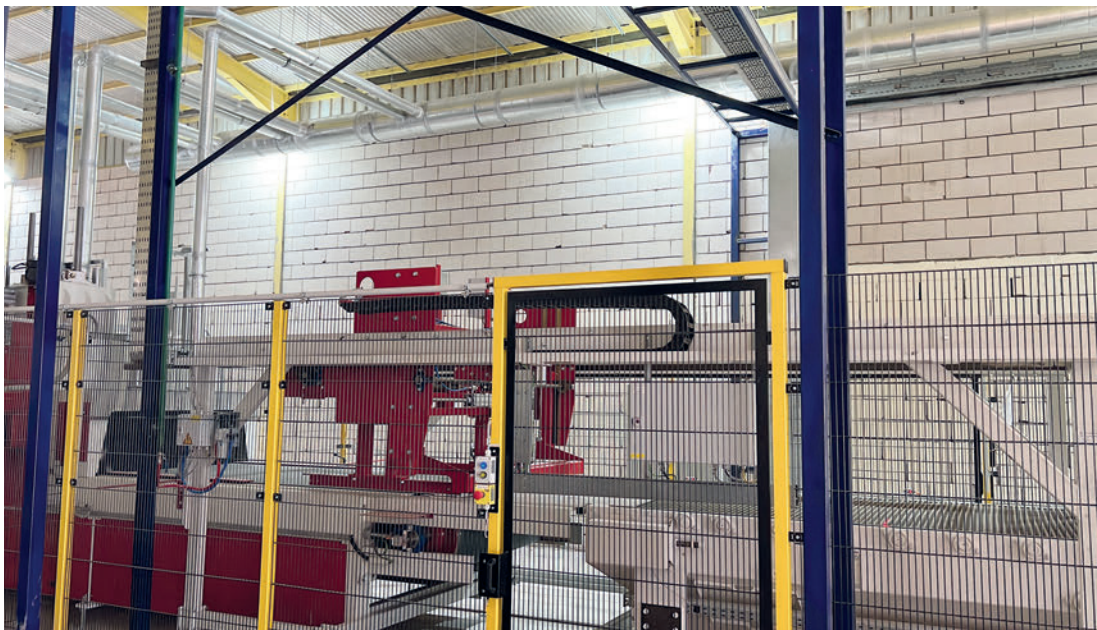
Layer pusher and retarder roller conveyor
