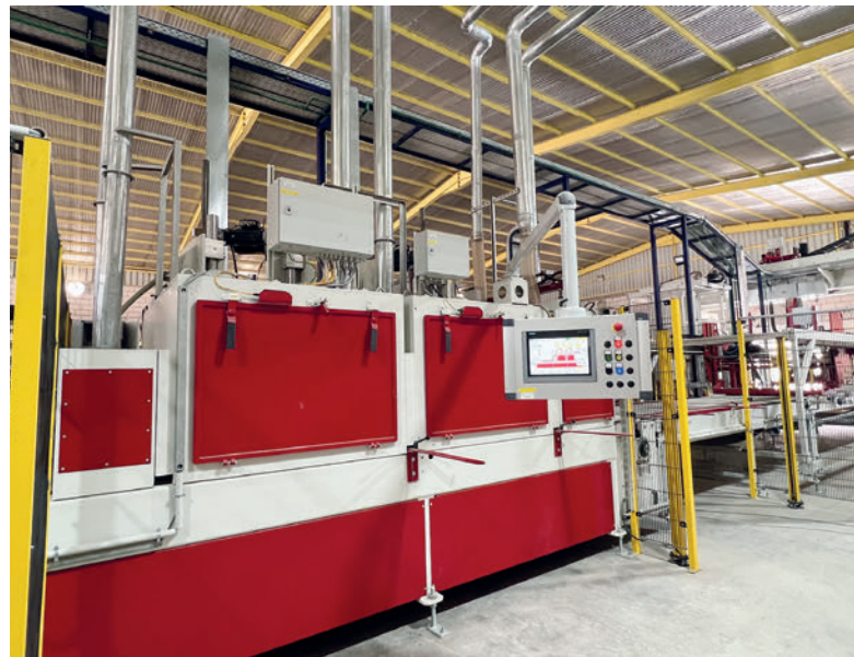
Curling machine with operation panel
