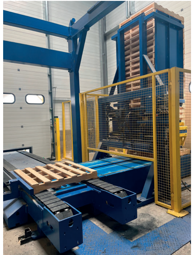
The pallet magazine is loaded from the outside, which is easy and safe.
