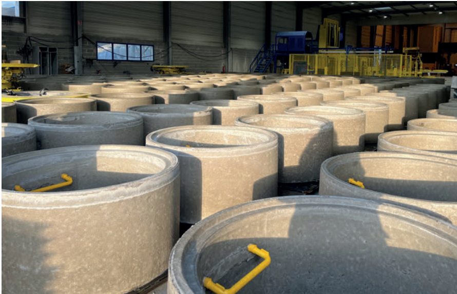
Manhole risers for sewage, with step rungs and anchors
