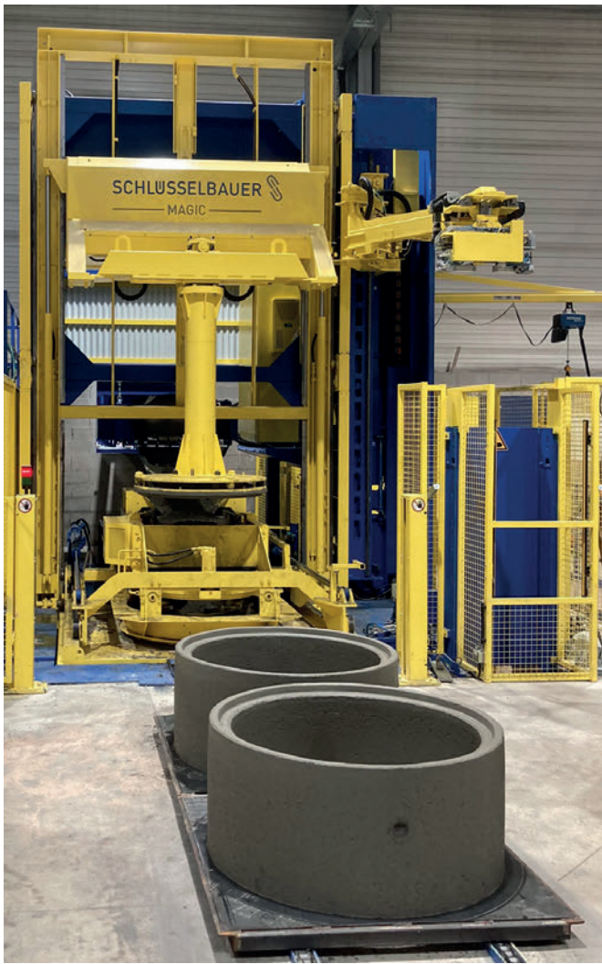
Anchors and step rungs are automatically positioned on the right of this photo, while the silo is offset behind the building wall. The Magic system was customized to fit the existing building.
