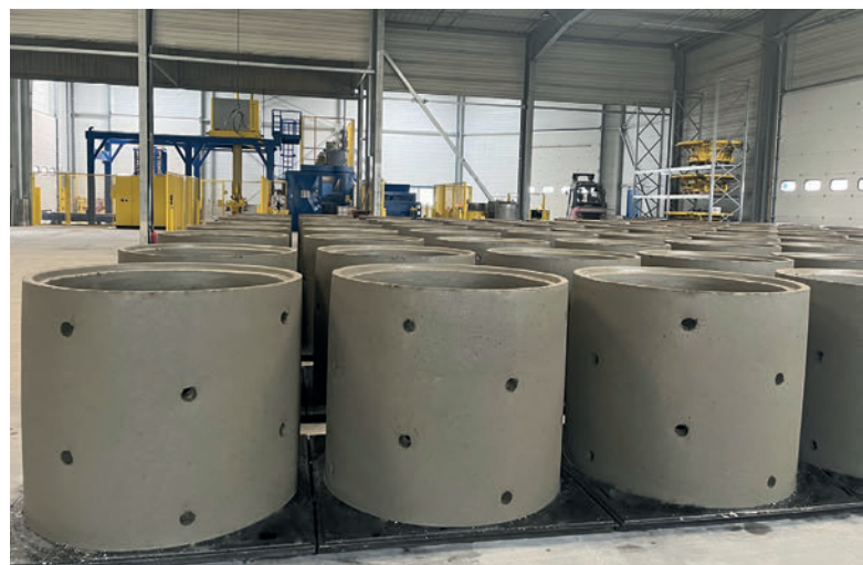
Optimum location of the curing area (here with manhole rings with drainage holes for rain water) in the hall between the production machine and palletizing system.
