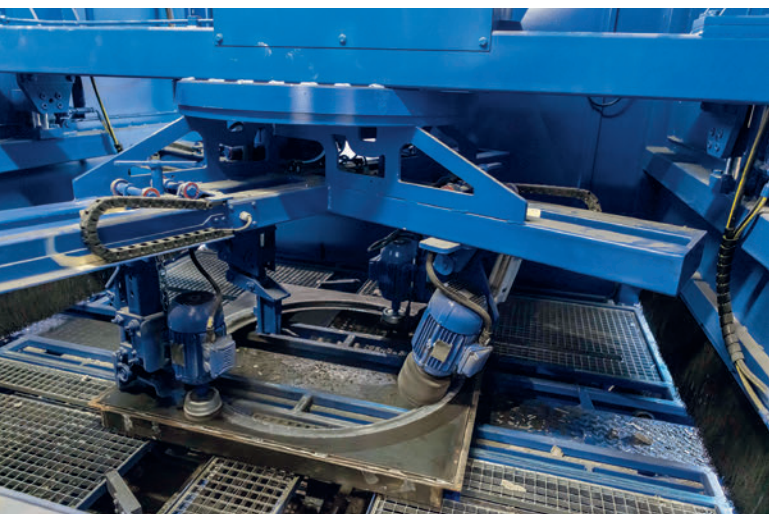
Cleaning station for bottom pallets, which is a key feature of Schlüsselbauer palletizing systems, along with spray-free oiling stations.
