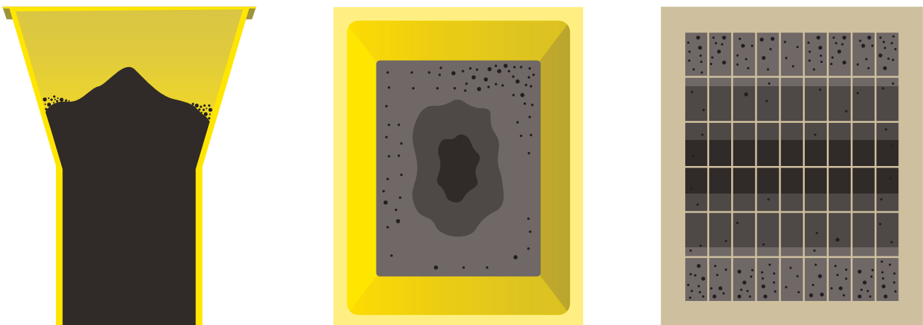
Section through the machine silo, top view machine silo, top view mould: Unfavourable distribution of the fresh concrete in the silo of the block making machine or on the production board.
