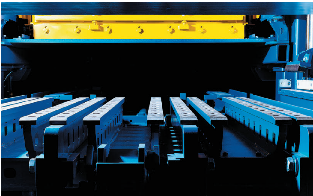
One-piece vibration table with vibrating elements and impact bars
