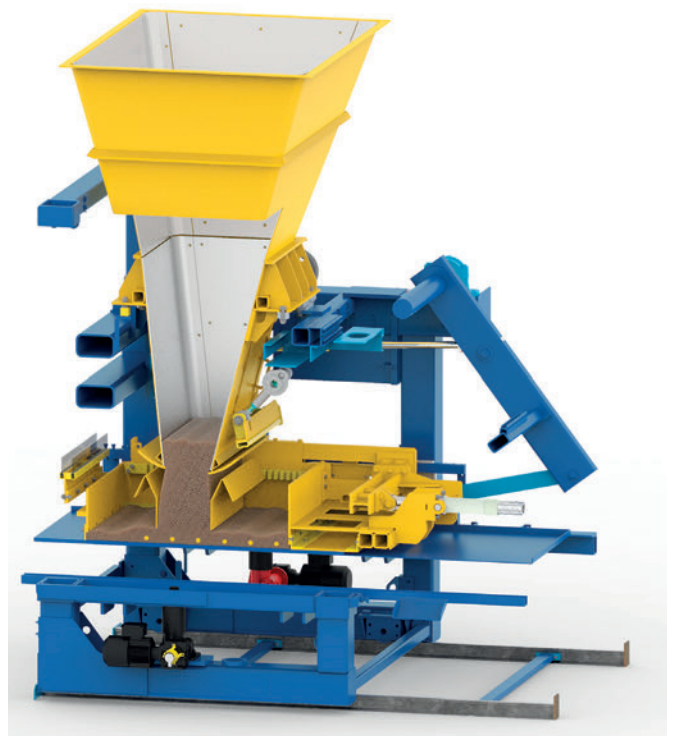
The number, length and positioning of the dosing angles have a direct effect on the material flow and thus enable exact dosing and repeatability.
