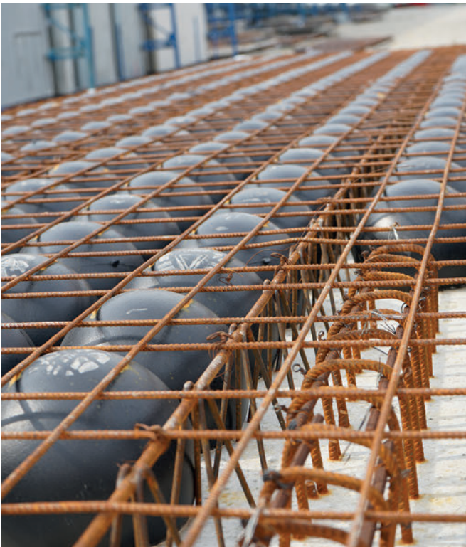
One of the main products and best seller of IJM is the bubbledeck slab.
